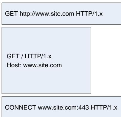
An intercepting transparent proxy receives this request from the client. Upon further inspection it identifies [www.site.com](http://www.site.com) in the HTTP request URI or Host header as the end destination host.
